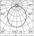
Luminous flux luminaire 4150 lm
