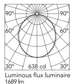
Beam Angle: 103° h(m) E(Ix)D(m) 638 2.54 2 160 5.07 3 71 7.61 4 40 10.14 5 26 12.68
