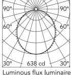
Beam Angle: 103° h(m) E(Ix)D(m) 638 2.54 2 160 5.07 3 71 7.61 4 40 10.14 5 26 12.68
