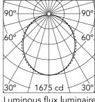
Beam Angle: 103° h(m) = E(Ix)D(m) 1675 2.54 2 419 5.07 3 186 7.61 105 10.14 5 67 12.68
