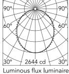
Beam Angle: 103° h(m) E(Ix)D(m) 2644 2.54 2 5.07 661 3 294 7.61 4 165 10.14 5 106 12.68
