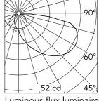
Luminous flux luminaire 212 lm
