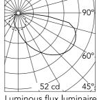
Luminous flux luminaire 212 lm
