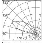
Luminous flux luminaire 2676 lm
