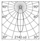
Luminous flux luminaire 860 lm
