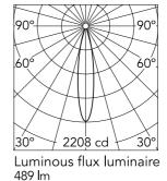
Beam Angle: 19° h(m) = E(Ix)D(m) 2208 0.34 552 0.67 3 245 1.01 4 138 1.34 88 1.68
