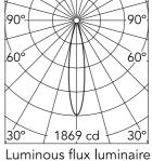
Beam Angle: 19° h(m) = E(Ix)D(m) 1869 0.34 467 0.67 3 208 1.01 4 117 1.34 75 1.68
