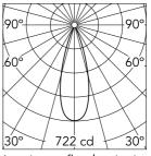
Luminous flux luminaire 364 lm
