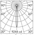
Luminous flux luminaire 479 lm
