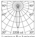
Luminous flux luminaire 489 lm
