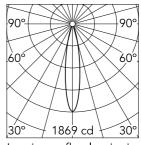
Luminous flux luminaire 414 lm
