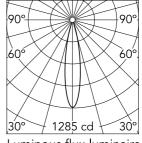
Luminous flux luminaire 193 lm
