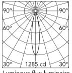
Luminous flux luminaire 193 lm
