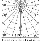
Luminous flux luminaire 314 lm
