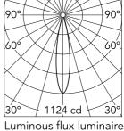
Beam Angle: 20° h(m) = E(Ix)D(m) 1124 0.35 281 0.70 3 125 1.06 4 70 1.41 45 1.76
