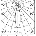
Luminous flux luminaire 170 lm (EXTREME CUT OFF)
