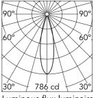
Luminous flux luminaire 170 lm (EXTREME CUT OFF)
