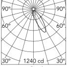
Luminous flux luminaire 770 lm (EXTREME CUT OFF)
