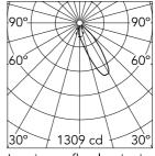
Luminous flux luminaire 682 lm (EXTREME CUT OFF)
