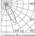
Luminous flux luminaire (EXTREME CUT OFF) 884 lm
