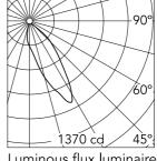
Luminous flux luminaire (EXTREME CUT OFF) 906 lm
