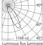
Luminous flux luminaire 964 lm (EXTREME CUT OFF)
