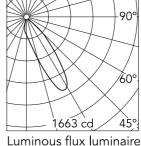
Luminous flux luminaire 828 lm (EXTREME CUT OFF)
