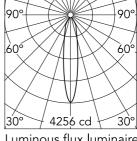
Luminous flux luminaire 1011 lm (EXTREME CUT OFF)
