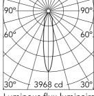
Luminous flux luminaire 1050 lm (EXTREME CUT OFF)
