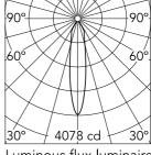
Luminous flux luminaire 1079 lm (EXTREME CUT OFF)
