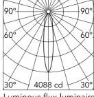
Luminous flux luminaire 955 lm (EXTREME CUT OFF)
