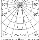
Luminous flux luminaire 869 lm (EXTREME CUT OFF)
