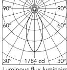
Luminous flux luminaire 976 lm (EXTREME CUT OFF)
