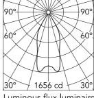
Luminous flux luminaire 960 lm (EXTREME CUT OFF)
