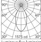
Luminous flux luminaire 1017 lm (EXTREME CUT OFF)
