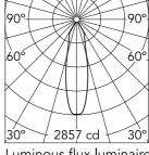
Luminous flux luminaire 895 lm (EXTREME CUT OFF)
