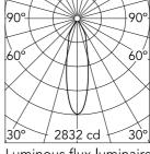
Luminous flux luminaire 1009 lm (EXTREME CUT OFF)
