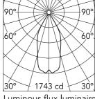
Luminous flux luminaire 996 lm (EXTREME CUT OFF)
