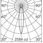
Luminous flux luminaire 632 lm (EXTREME CUT OFF)
