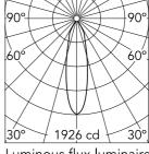
Luminous flux luminaire 594 lm (EXTREME CUT OFF)
