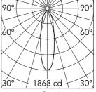
Luminous flux luminaire (EXTREME CUT OFF)
