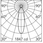
Luminous flux luminaire 637 lm (EXTREME CUT OFF)
