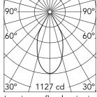
Luminous flux luminaire 729 lm (EXTREME CUT OFF)
