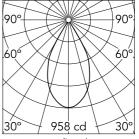
Luminous flux luminaire 622 lm (EXTREME CUT OFF)
