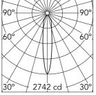
Luminous flux luminaire 629 lm (EXTREME CUT OFF)
