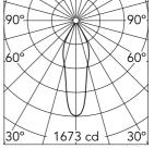
Luminous flux luminaire 663 lm (EXTREME CUT OFF)
