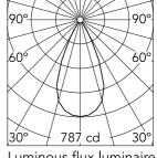
Luminous flux luminaire 511 lm (EXTREME CUT OFF)
