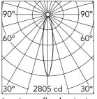
Luminous flux luminaire 740 lm (EXTREME CUT OFF)
