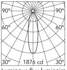
Luminous flux luminaire 641 lm (EXTREME CUT OFF)
