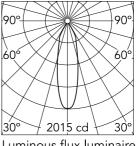
Luminous flux luminaire 735 lm (EXTREME CUT OFF)
